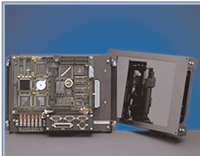
**WinSystems' Panel PC puts all the pieces together in a compact, rugged form for use as a display subsystem for factory automation or industrial instrumentation, including a flat panel VGA display, SBC with Ethernet and PC/104 expansion, plus optional touch screen.**
